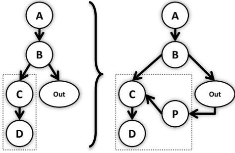
**Figure 10:** The post-computation transformation. P represents a `postcompute` node.
